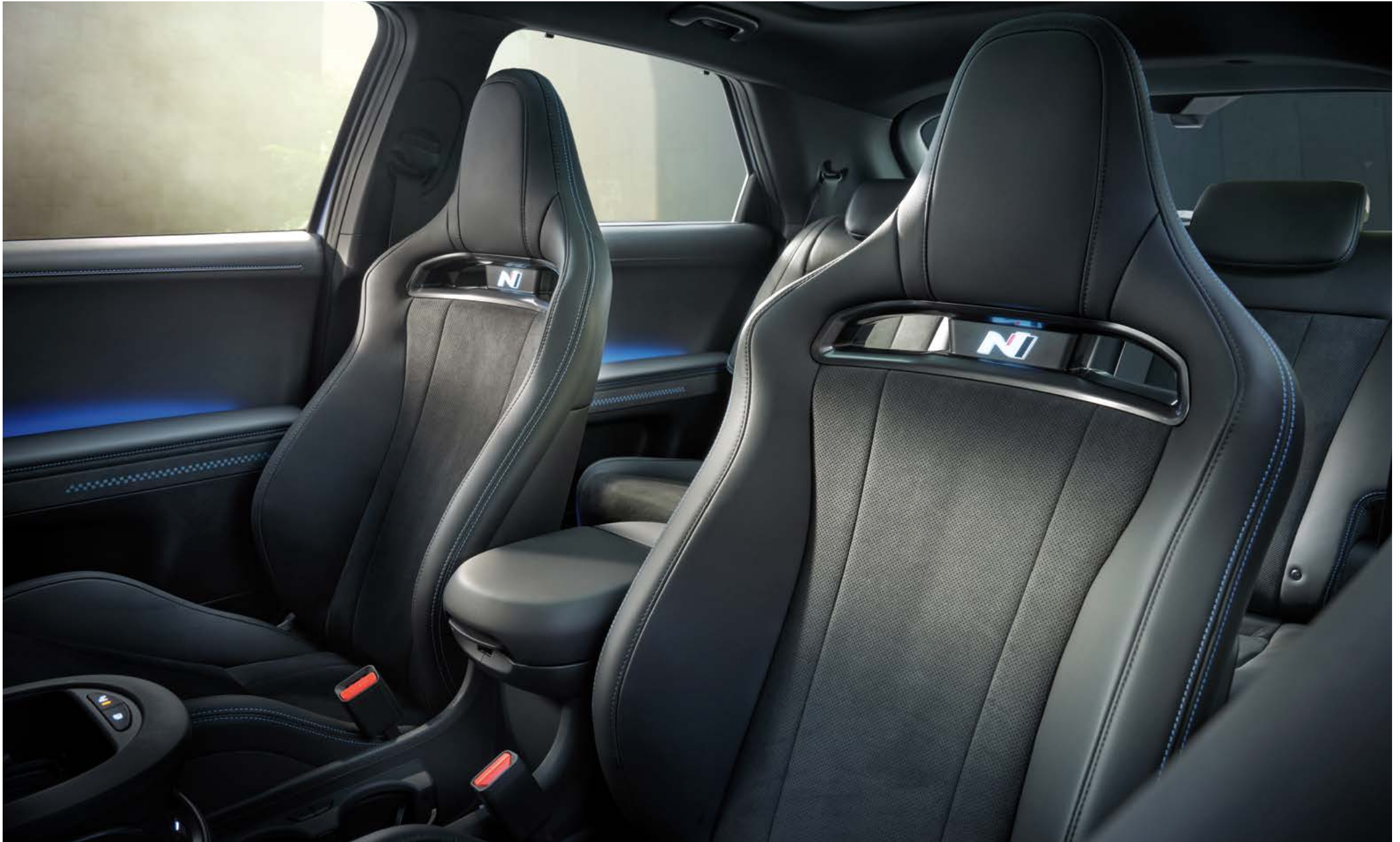
The N Light sports bucket seats feature mixed Alcantara suede/natural leather, built-in headrests, heated/ventilated seats, and the N logo on the front/rear(front lighting).
