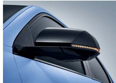
Black outside mirror (heating, power-folding, power adjustment, LED turn signal lamps)
