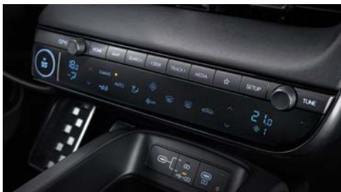
Dual-zone full automatic air conditioning(with micro air filter, auto defog system, fine dust sensor, air cleaning mode, and after-blow function)
