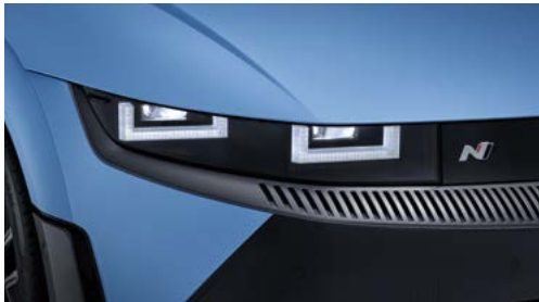
Full LED headlamps(projection type), LED DRL & turn signal lamps
