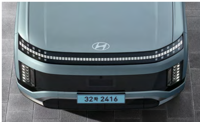
Small-Cube Projection Led Headlamps (Daytime Lights, Positioning Lamps, Turn Signals)
