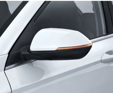
LED headlamps (MFR type) Side mirrors (heated, power-folding, power-adjustable, LED turn signal indicators)
