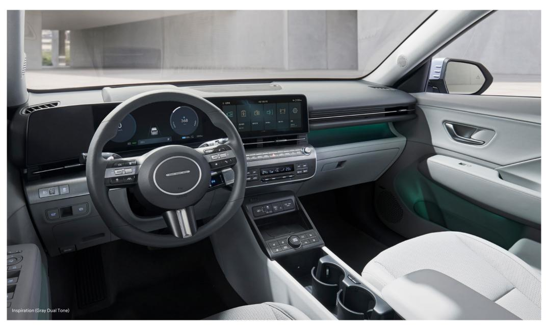
Panoramic display (12.3-inch LCD cluster, 12.3-inch navigation), ambient mood lighting, dual full-auto air conditioning with micro-air filter/auto-defog/dust sensor/air quality mode/after-blow \*\* Range per charge may vary by trim and options.
