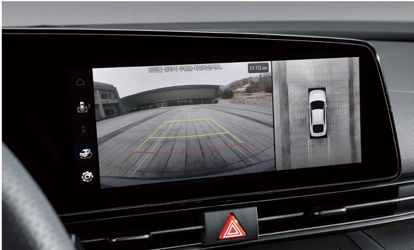
Surround View Monitor For safe parking, the surround view monitor shows the situation around the vehicle in crystal-clear image quality by applying a high-definition camera and digital video transmission method.
