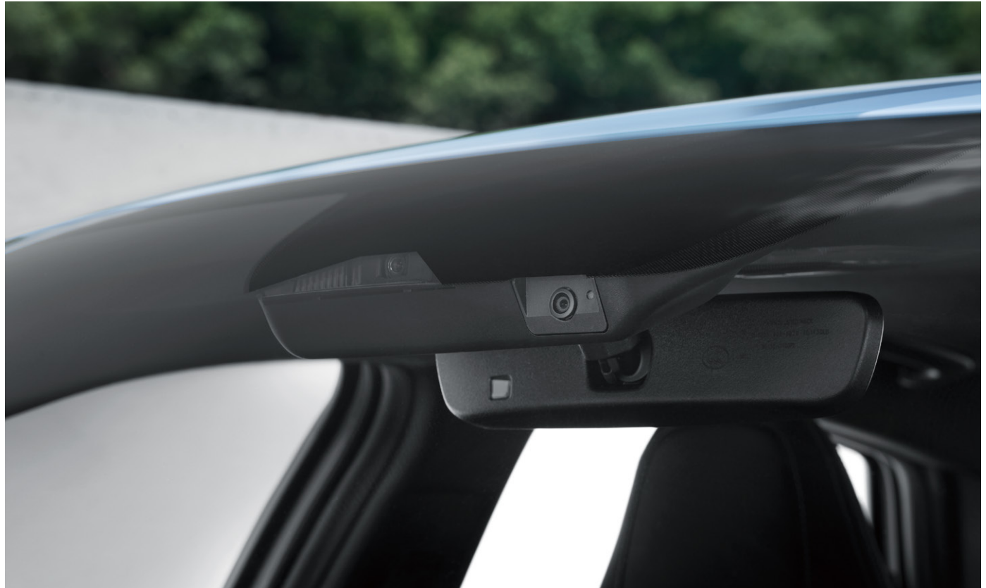
Built-in Camera A built-in high-resolution dash cam allows recorded footage to be viewed on the AVN screen or shared on social media via smartphone app integration.
