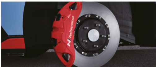
N Performance Brake System (Monoblock 4-piston calipers, bolt-on hybrid discs)
