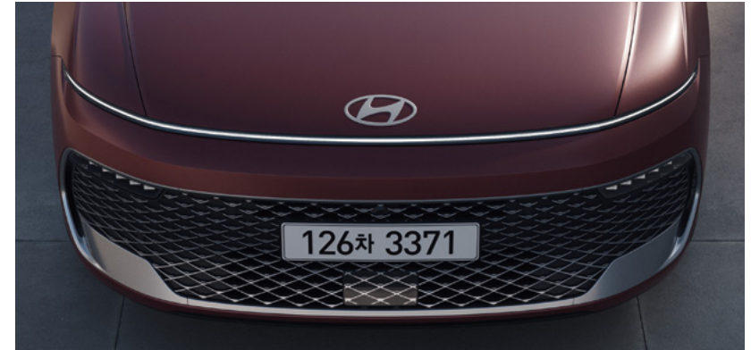
Horizontal LED lamp (Seamless Horizon Lamp - daytime running lights, turn signals, positioning lamps)
