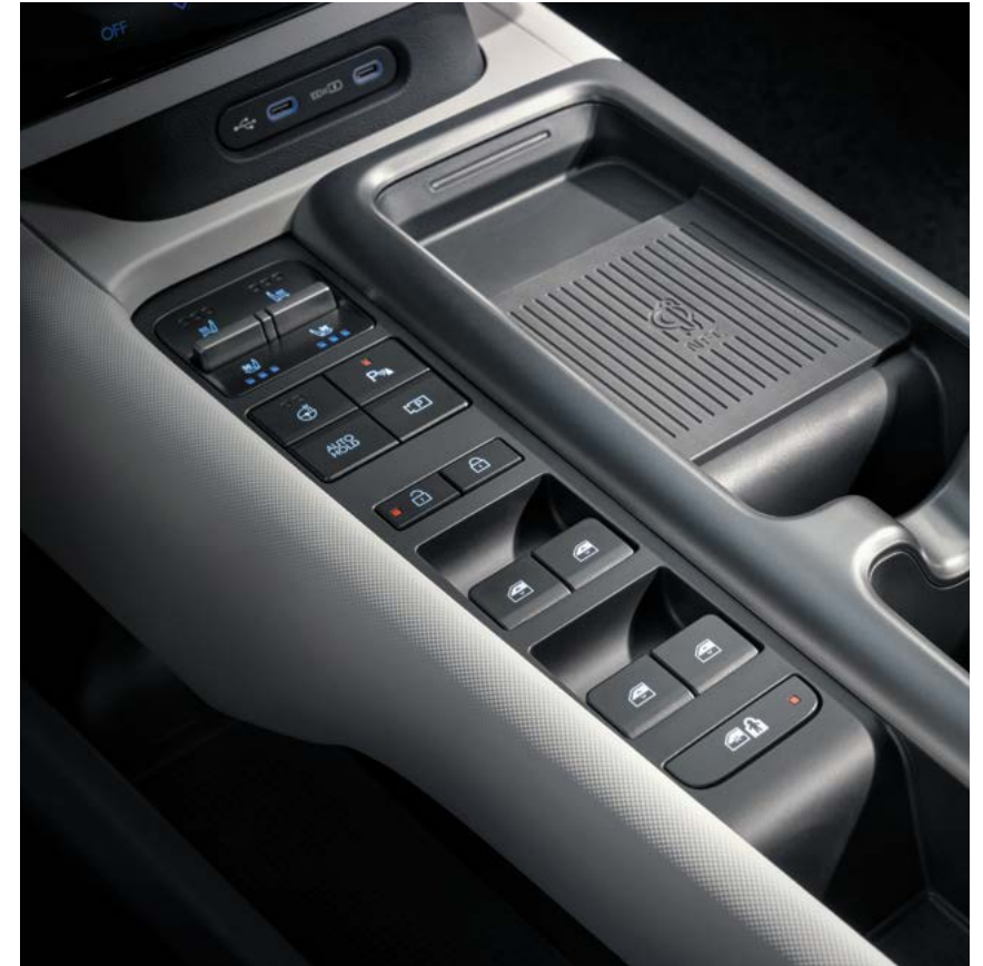
Console switch (windows, ventilation, heating)
