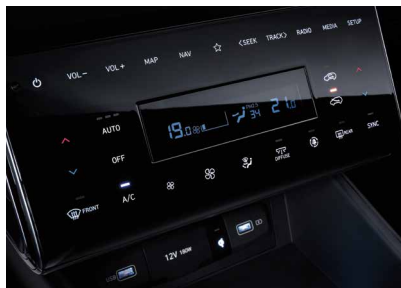
Roof rack Dual-zone full automatic air conditioning (with auto defog system, fine dust sensor, air cleaning mode, multi-air mode, and after-blow function)
