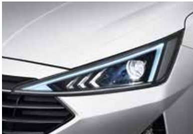
Projection headlamps(bi-function) & Bulb daytime running lights(DRL) Projection headlamps(bi-function) & LED daytime running lights(positioning lamps)
