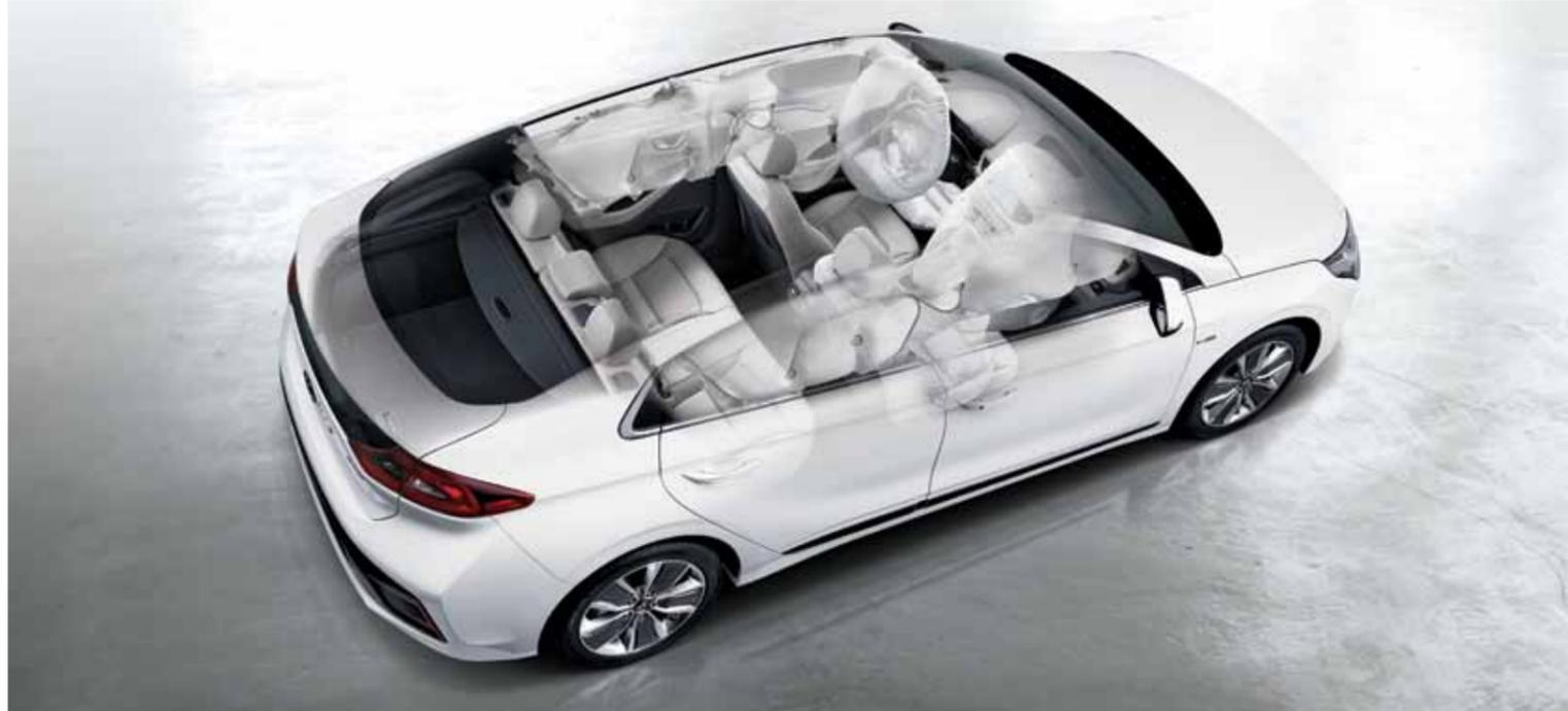
Seven-airbag system (advanced frontal airbags, driver's knee airbag, driver and front passenger side airbags, and curtain airbags)
