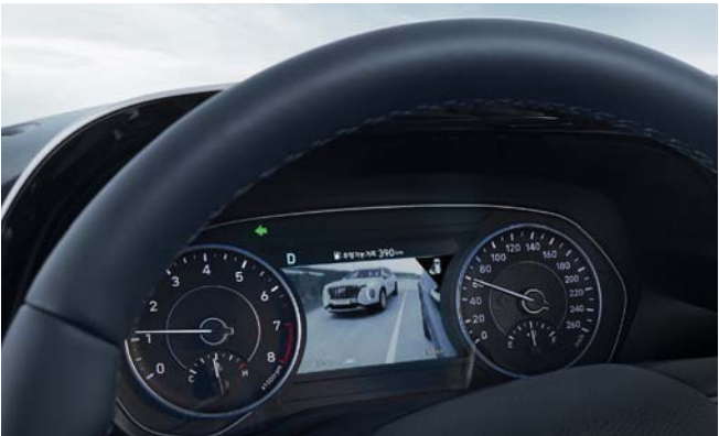
Driver Attention Alert The Palisade continuously conducts a comprehensive analysis of the driver's driving patterns, the position of the car within the lane, and other relevant information. If the vehicle detects that the driver is struggling with exhaustion or driving carelessly, a warning sound and pop-up message recommending that the driver take a rest are issued.
