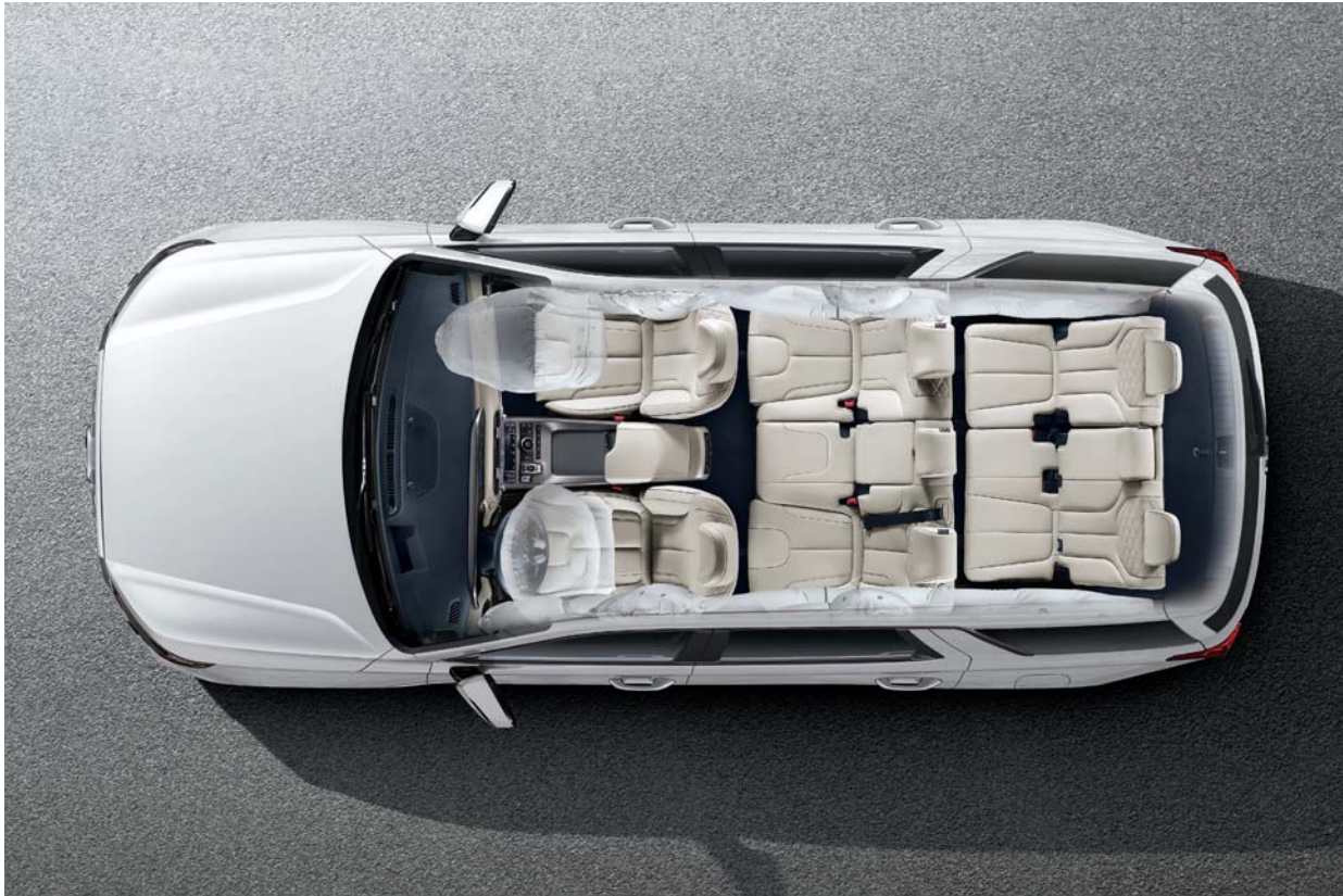
9 airbag system The Palisade offers nine airbags, including curtain airbags that protect passengers in all seats, airbags for the driver's and front passenger seats, side airbags between the front- and second-row seats, and a knee airbag for the driver.
