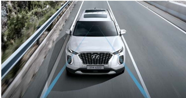
Forward Collision Warning / Forward Collision-avoidance Assist This function warns the driver in cases of impending collision with the vehicle in front. When necessary, it helps prevent a collision by taking control of the vehicle's brakes.
