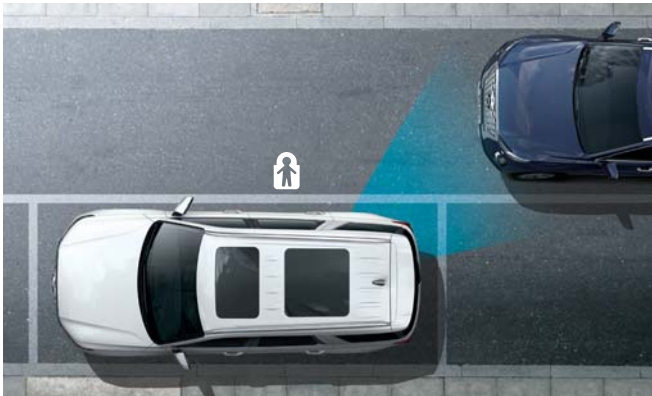
Blind-spot Collision Warning / Blind-spot Collision-avoidance Assist This function alerts the driver of vehicles approaching from the rear or that are positioned in the vehicle's blind spots. When necessary, this function takes control of the vehicle's brakes to prevent rear/blind-spot collision.
