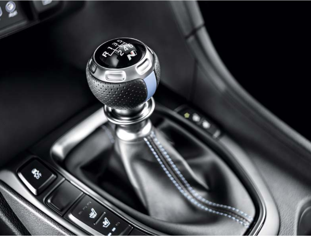
N-exclusive 6-speed manual transmitter and rev matching system The rev matching system that synchronizes RPM during speed shifting works to minimize any possible shock from speed shifting and provides dynamic transmission.
