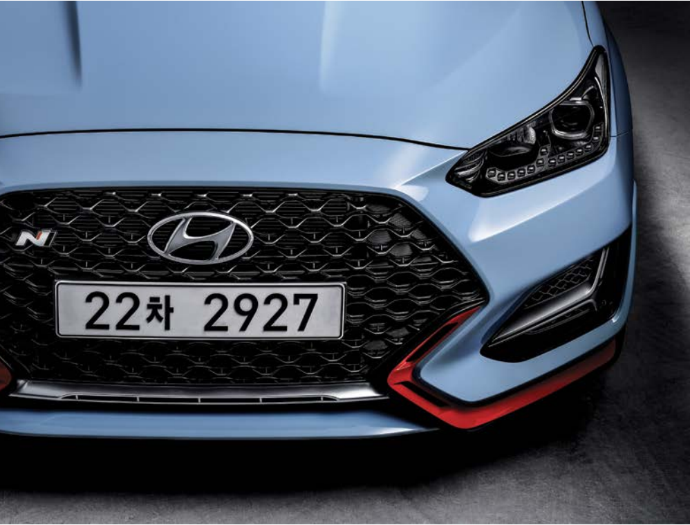
Wide-type radiator grille and air curtains The glossy black, wide radiator grille adds a sporty feel and enhances the air conditioning function, while the wing-shaped, external air curtains improve the aerodynamics.
