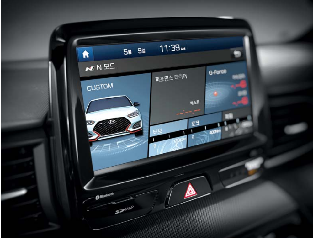
N Grin Control System The N Grin Control System adjusts powertrain and chassis settings based on driving preferences and road conditions and measures output, torque, and acceleration of gravity in real time.
