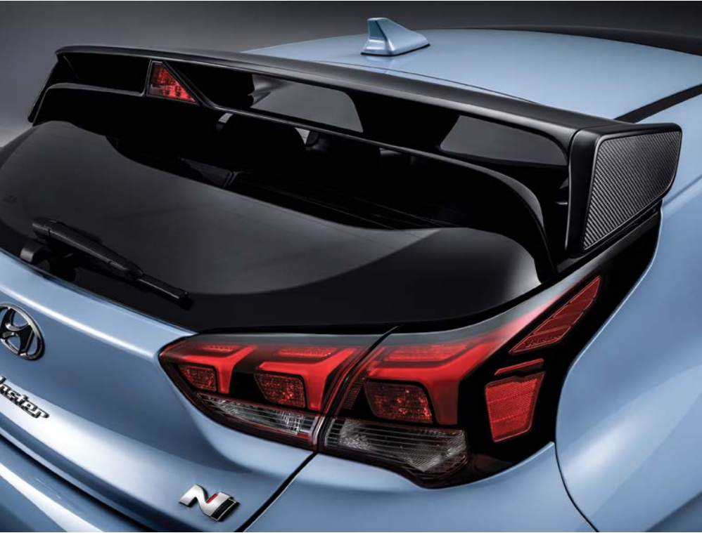
Wing-type rear spoiler The wing-type rear spoiler elevates the aerodynamics of this high-performance hatch to new heights, and a high-mounted brake light is installed at the center of the rear spoiler to ensure safe driving.
