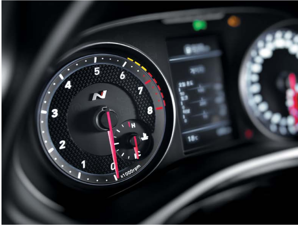
4.2-inch supervision cluster The supervision cluster applied with the N logo adds to the fun driving experience and informs the driver of the exact timing for shifting.
