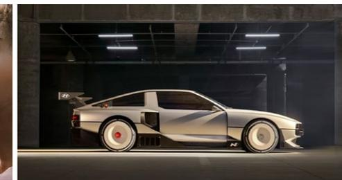
N Vision 74- high-performance hydrogen fuel cell-hybrid "Rolling Lab"
