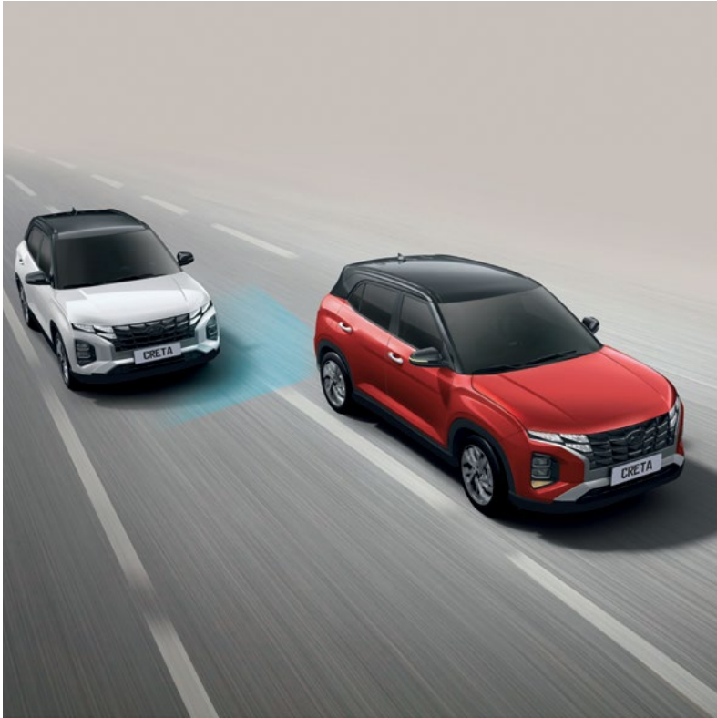
Blind-spot Collision-Avoidance Assist (BCA) BCA monitors your blind spot while driving. When a vehicle is detected in the vicinity of your car, the LED on the rearview mirror will light up, giving a warning and automatically braking if needed.
