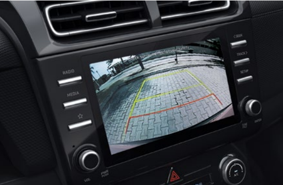
Rear View Monitor (RVM) RVM makes sure it is safer when reversing or parking. The rear camera will monitor the rear area of the car.
