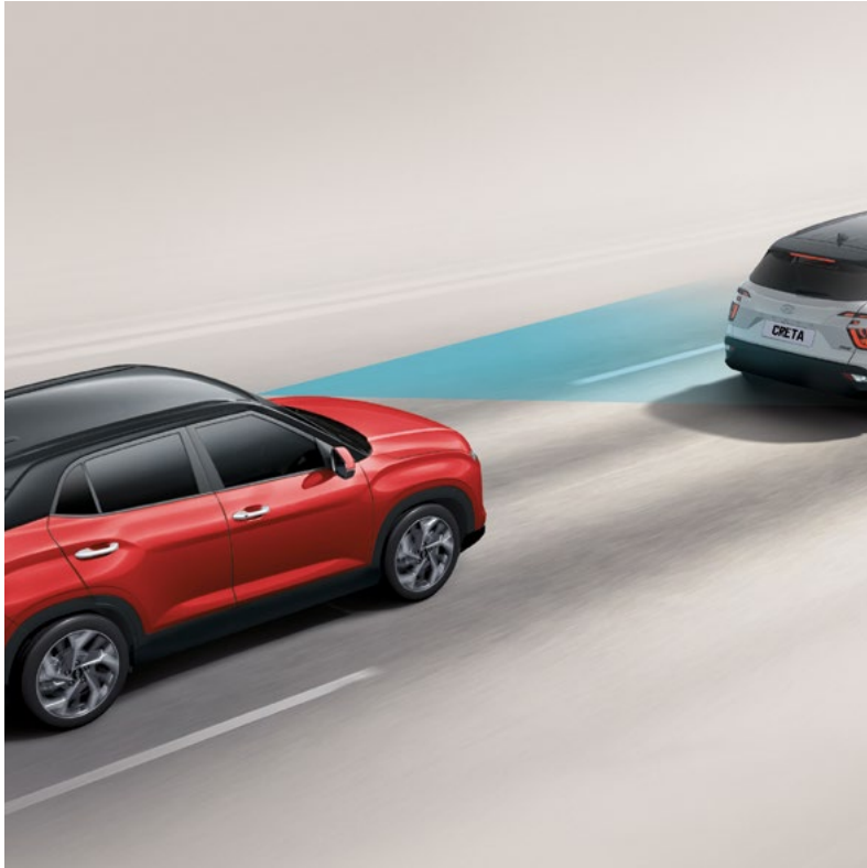
Forward Collision-Avoidance Assist (FCA) This feature warns the driver when the system detects a risk of a front-end collision such as with pedestrians or a vehicle that suddenly slows down or stops. If the collision risk increases after the warning, the system will automatically assist by applying emergency braking.
