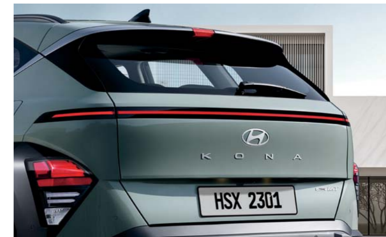
Spoiler Integrated HMSL, rear seamless horizon lamp LED brake lamps, LED turn signal lamps
