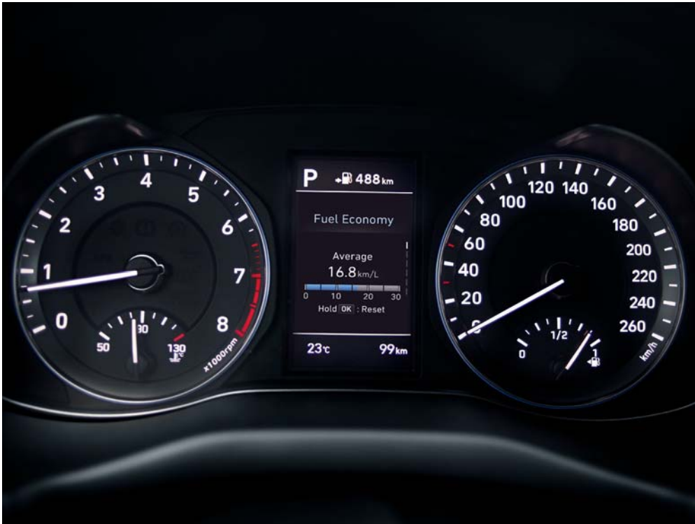
Digital Information Cluster Optimally placed and easy to read, a 4.2" LCD screen shows you important driver information like: the status of active safety features, remaining range and fuel consumption, navigation instructions, outside temperature and more.
