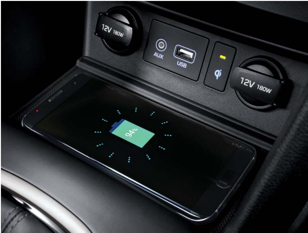
Wireless phone charging Ocated in the centre console, a wireless charging pad (Qi standard) lets you easily charge a compatible Qi - enabled smartphone without the use of messy and unsightly cables.
