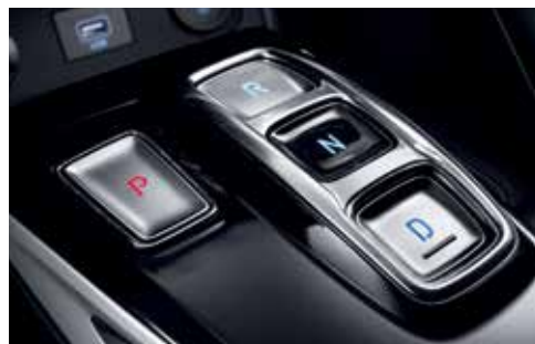
Shift-by-wire automatic transmission
