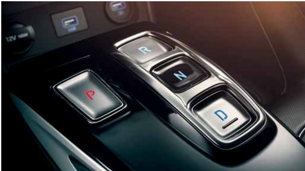
Shift-by-wire automatic transmission
