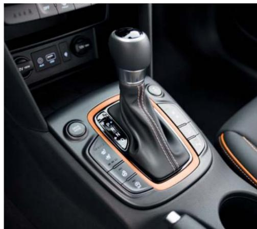
7-speed dual-clutch transmission (DCT)
