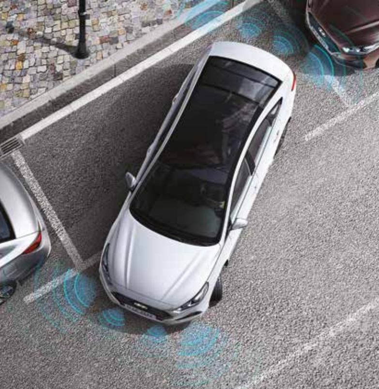
Parking Assist System (PAS) Sensors at the front and rear assist safe parking by activating an audible warning if you get too close to objects when reversing.
