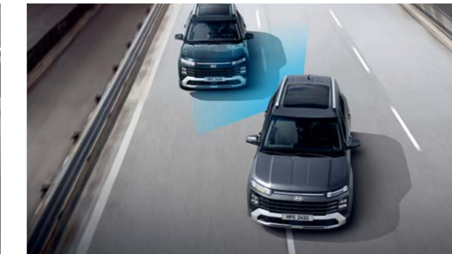
Blind-Spot Collision-Avoidance Assist (BCA) Blind-Spot Collision-Avoidance Assist (BCA) warns you if there is a risk of collision with a rear side vehicle in the blind-spot while changing lanes. When forward exiting a parallel-parking spot, if there is a risk of collision with a vehicle approaching from behind, it automatically assists with emergency braking.
