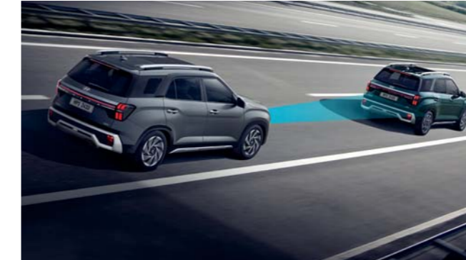
Smart Cruise Control with Stop & Go (SCC with S&G) Smart Cruise Control (SCC) helps maintain distance from the front vehicle and drive at a speed set by the driver. Automatically stops when the front vehicle stops and automatically starts when the front vehicle departs within a short time.
