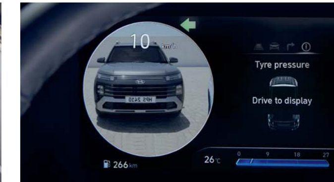
Blind-Spot View Monitor (BVM) When the turn signals are activated, the rear-side image of the corresponding direction is displayed in the cluster.
