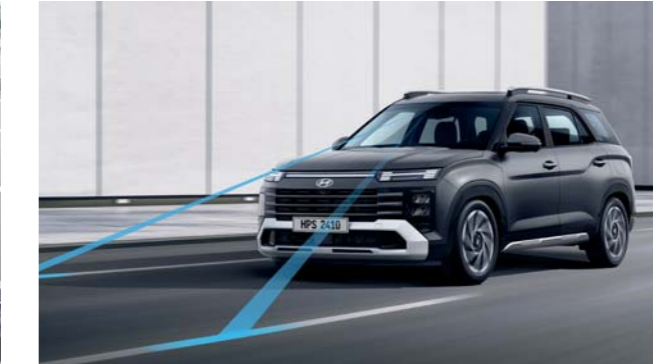
Lane Keeping Assist (LKA) If driving above a certain speed and the driver leaves a lane without the turn signal switch being operated, it provides a warning. When a lane departure is detected, it automatically assists with steering to help prevent leaving the lane.
