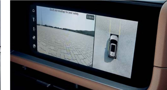
Surround View Monitor (SVM) Surround View Monitor (SVM) displays images of the situation around the vehicle in various views for safe parking.
