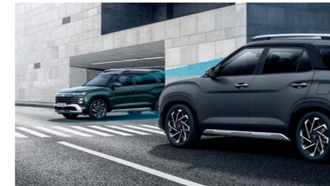
Forward Collision-Avoidance Assist 1.5 (FCA 1.5) Alerts the driver if the vehicle ahead is slowing down too quickly or if there is the potential for a forward collision with stationary vehicles, pedestrians, cyclists ahead, or approaching vehicles on the road, and activates the brakes in the event of an impending collision. Forward Collision-Avoidance Assist also brakes automatically to avoid an impending collision with vehicles or cyclists ahead on the road or approaching from either side while making a left turn at an intersection.
