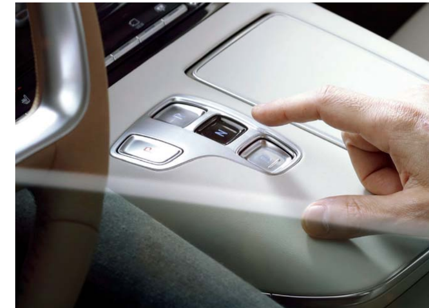
Shift-by-wire automatic transmission
