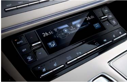
Touch-screen climate controller (Dual automatic A/C)
