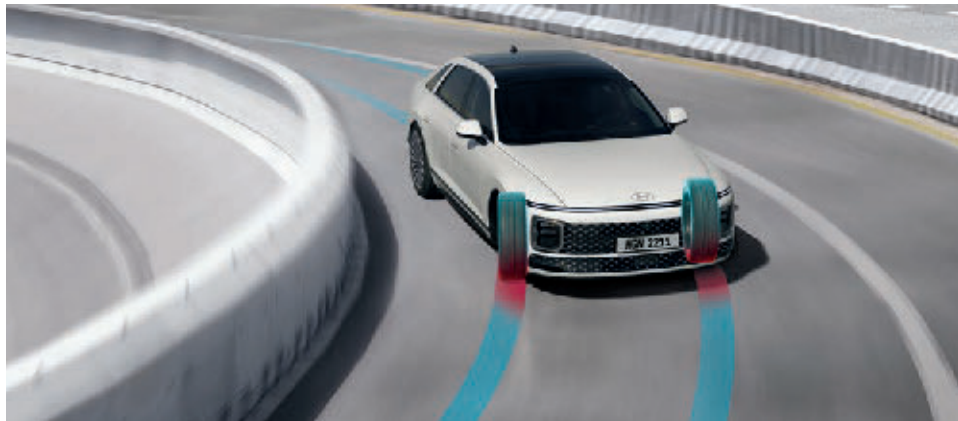
When the vehicle approaches a turn, the hybrid system regulates the vehicle's movement to execute torque vectoring while simultaneously maintaining the ideal level of tire grip for dynamic handling performance.
