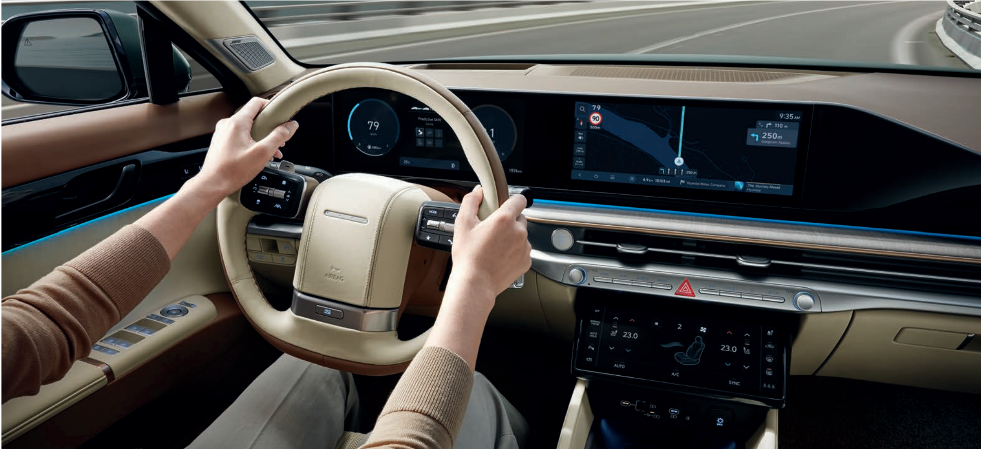
Predictive Gear-shift System (PGS) Improves driving safety and comfort by predicting acceleration/deceleration conditions and shifting to the optimum gear in combination with ADAS navigation and radar signals.
