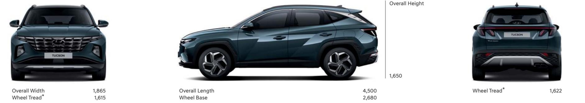
Unit : mm \* Wheel tread • 17" Wheel (Front/Rear) : 1,630/1,637 • 18" Wheel (Front/Rear) : 1,615/1,622 • 19" Wheel (Front/Rear) : 1,615/1,622
