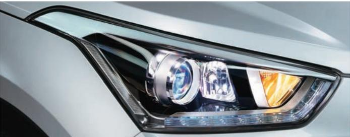
Bi-functional Projector Headlamps with LED Positioning Lamps
