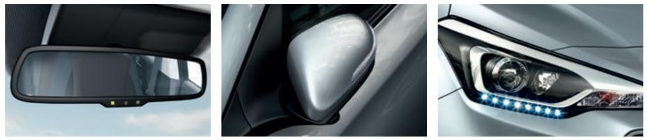
Electro-chromatic mirror (ECM). The interior mirror automatically darkens when its sensor detects glare from the headlights of following vehicles.
