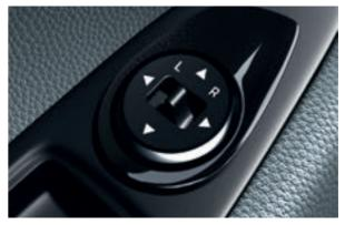
**Powered and heated door mirrors.** The door mirrors can be remotely adjusted and heated from the door console.
