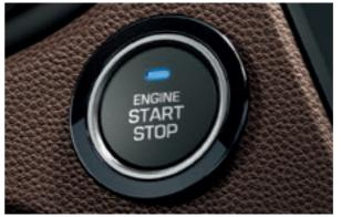
Engine start/stop button. Keyless starting when the smart key is on board in your pocket or bag.
