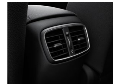
Rear air ventilation system
