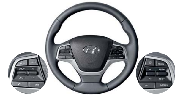
Steering wheel includes remote control functions for audio, cruise control and Bluetooth
