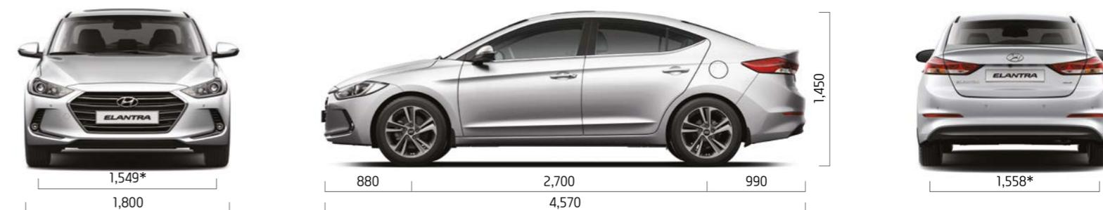
\* Wheel tread • 15" alloy wheels (Front/rear) : 1,563/1,572 • 16" alloy wheels (Front/rear) : 1,555/1,564 • 17" alloy wheels (Front/rear) : 1,549/1,558
