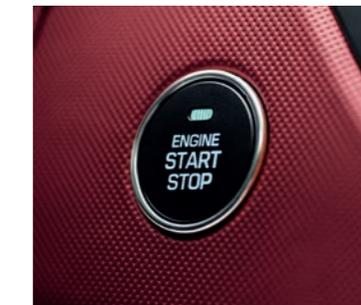
**Engine Start/Stop button.** When you're on board with the smart key in your pocket or in your bag, keyless push-button starting is enabled.
