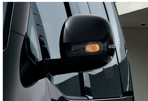
LED Turning Signal on Side Mirror
