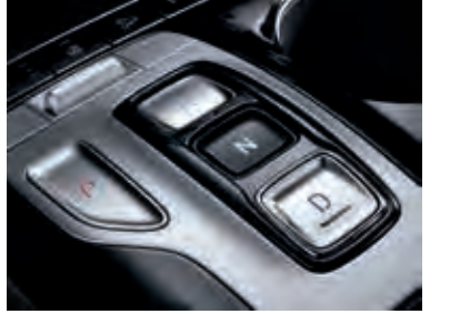
Elektronik vites paneli (Shift by Wire) (P / P+ / E / E+ / N)
