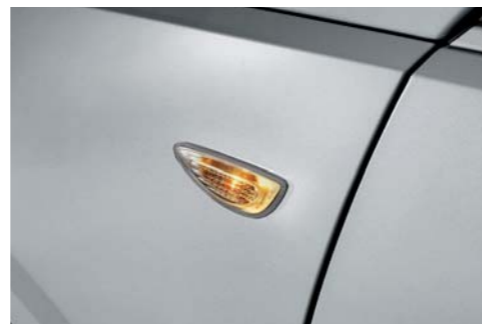
Fender turn signal (Bulb-type, STD)
