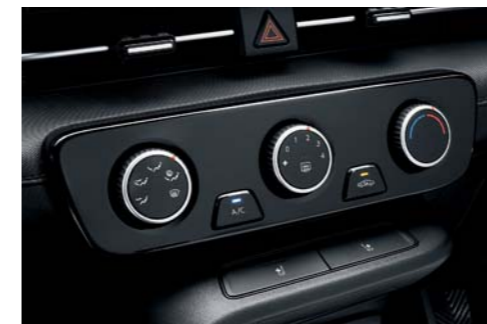
Manual air conditioning system
