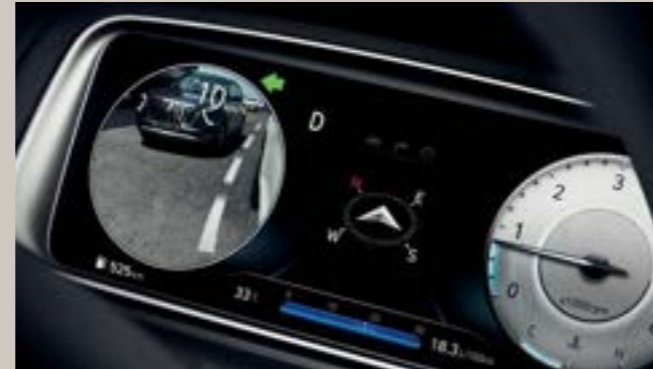
Blind-Spot View Monitor (BVM) When the turn signals are activated, the rear-side image of the corresponding direction is displayed in the cluster.
