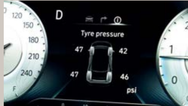
Tyre Pressure Monitor System (TPMS) TPMS helps you achieve optimal fuel economy and extends tire life by alerting you if the tires require attention.
