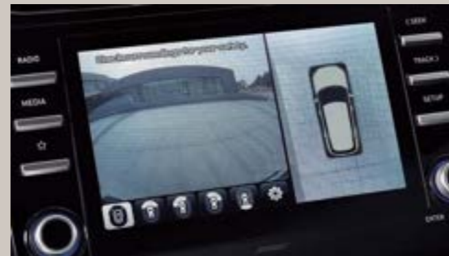
Surround View Monitor (SVM) A multi-camera system provides a 360-degree view around the vehicle to assist the driver in parking situations.
