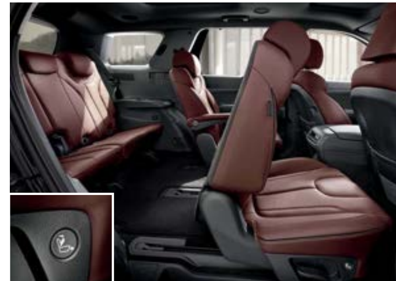
Smart one-touch walk-in (WALK-IN DEVICE(REAR))
