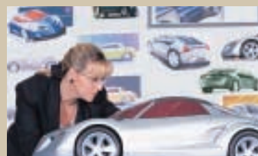
A new concept takes shape with a 1:4 scale clay model
