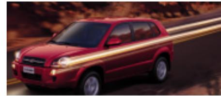
*Tucson uses the state-of-the-art Borg-Warner Electronic InterActive Torque Management four-wheel-drive system that routes up to 99 percent of the available power to the front wheels. As road conditions or torque demand changes, the system automatically diverts up to 50 percent of the available power to the rear wheels. The system monitors throttle position, front wheel angle and slippage.*
