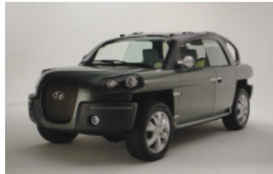
The OLV is powered by a 2-liter four-cylinder DOHC engine but with the help of a Borg-Warner supercharger and intercooler system, manages to generate up to 150 kW for some adrenalin pumping fun.
