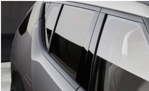
Acoustic Laminated Glass (rear & front)
