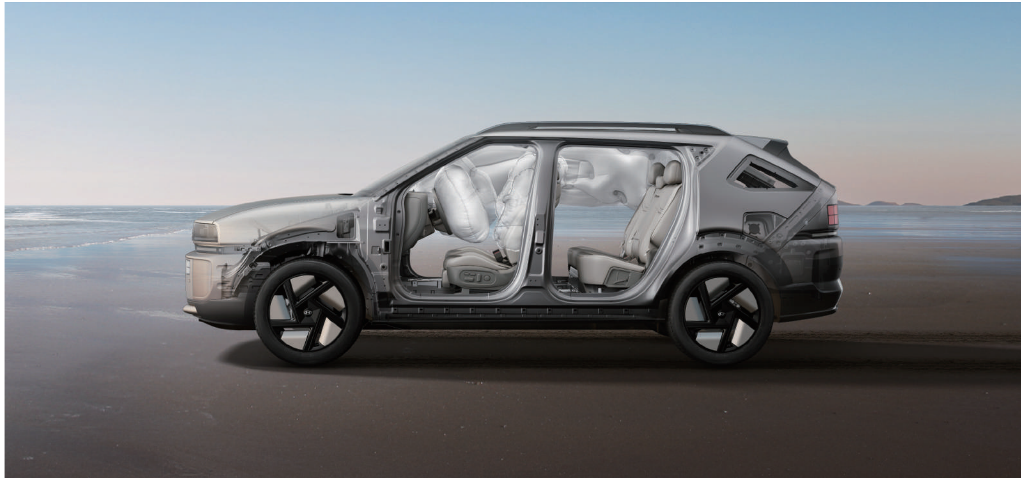
Platform Reinforcement & 7-Airbag System
