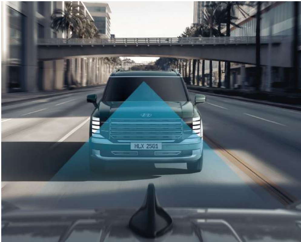
Smart Cruise Control (SCC) Smart Cruise Control (SCC) helps maintain distance from the front vehicle and drive at a speed set by the driver. Automatically stops when the front vehicle stops and automatically starts when the front vehicle departs within a short time.
