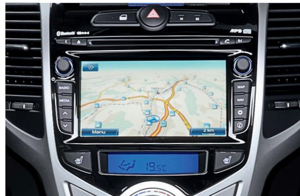
**New generation audio and navigation system.** The new audio system includes iPod connectivity, integrated My Music storage (1 GB) and AUX and USB ports. The navigation system has a 6.5" TFT colour touch screen that also functions as the display for the integrated rear view camera.
