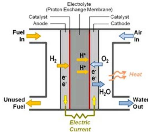
The fuel cell electrochemical process is as follows:
