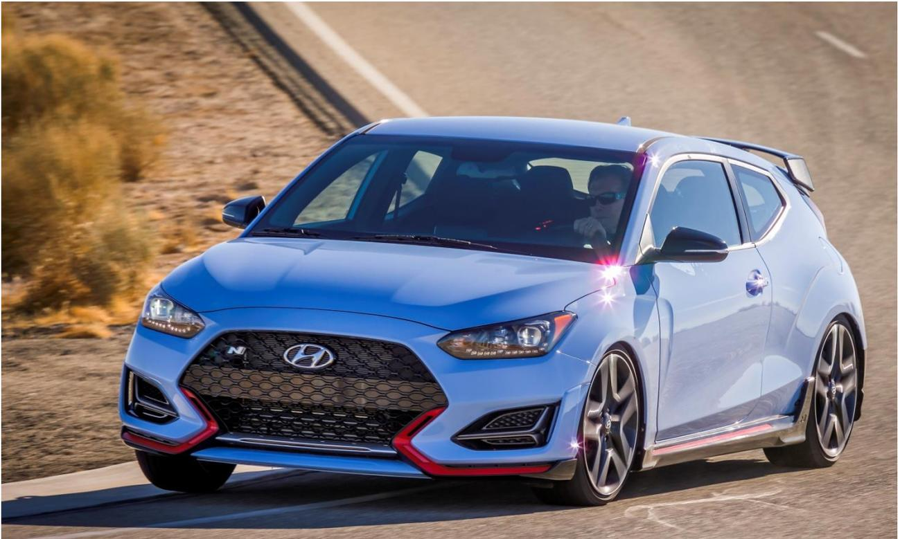
In profile, exclusive N-design rocker side sills and available lightweight 19-inch alloy wheels with a machined-finish dual-spoke star design clearly differentiate the N model from other Veloster models. Tires are of the ultra-high performance category, with standard 225/40R18 Michelin Pilot SuperSport summer tires for the 18-inch wheel design and exclusive-compound 235/35R19 Pirelli P-Zero summer tires for the available 19-inch alloy wheel.
