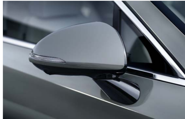
Full LED headlamp (projection type) / Chrome radiator grille Exterior mirror (LED repeater, heating, power adjustment, power-folding)
