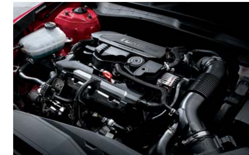
SONATA Sensuous_Smartstream Gasoline 1.6 Turbo engine
