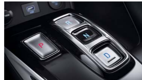
Double-glazed soundproof glass (front side, front doors) Shift By Wire
