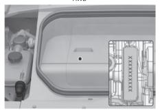
The motor numbers can be checked at the bottom of the vehicle.
