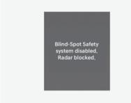
When the rear bumper around the rear corner radar or sensor is covered with foreign material, such as snow or rain, or installing a trailer or carrier, it can reduce the detecting performance and temporarily limit or disable Safe Exit Assist.
