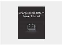
When the high voltage battery level reaches below about 10 %, this warning message is displayed.
