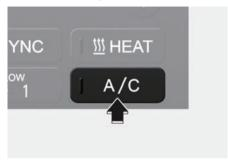
Touch the 'CLIMATE' icon in the climate control screen. The climate information screen will appear on the infotainment screen. Touch the A/C icon in the infotainment screen to turn the air conditioning on (indicator light ON) and off.
