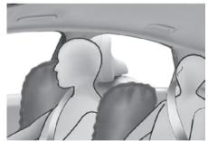
Your vehicle is equipped with a side airbag in each front seat. The purpose of the airbag is to provide the vehicle's additional protection than that offered by the seat belt alone.
