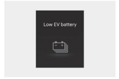
When the high voltage battery level reaches below about 20 %, this warning message is displayed.
