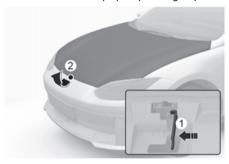
3. Go to the front of the vehicle, raise the hood slightly, push to the left the secondary hood release lever (1) inside of the hood center and lift the hood (2).
