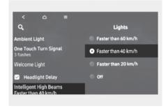
With the Start/Stop button in the ON position, select **Setup** > **Vehicle Settings** > **Lights** > **Intelligent or Smart High Beams** from the Settings menu to turn on Intelligent Front-Lighting System and deselect to turn off the system.
