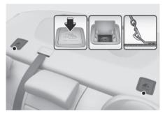
Top-tether anchorages for Child Restraint Systems are located on the rear of the seathacks
