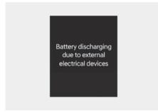
This warning message is displayed when a battery discharge due to excessive current is detected by mounting an unauthorized electrical device such as a black box.
