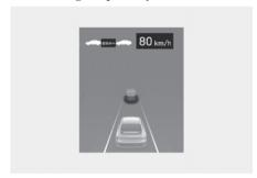
If you want to speed up temporarily without altering the set speed while Smart Cruise Control is operating, depress the accelerator pedal. While the accelerator pedal is depressed, the set speed, distance level and target distance will blink on the instrument cluster.
