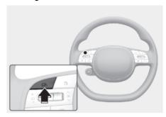
Press the Driving Assist ((-(-(-))) button to turn Cruise Control off. The Cruise ((\*(-(-(-)))) indicator will go off.
