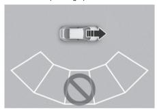
Remote Smart Parking Assist does not work properly when the parking lines are not parallel. Do not park although the parking space is recognized by the sensor.
