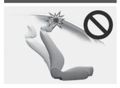
If you recline the seatback towards the front with the headrest and seat cushion raised, the headrest may come in contact with the sunvisor or other parts of the vehicle.
