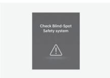
When Safe Exit Warning is not working properly, the 'Check Blind-Spot Safety system(s)' warning message will appear on the instrument cluster for several seconds, and the master (A) warning light will illuminate on the instrument cluster. If this occurs, we recommend that you have the vehicle inspected by an authorized HYUNDAI dealer.
