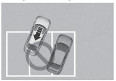
If Remote Smart Parking Assist is used when parking in a space next to misaligned vehicles, your vehicle may not be parked side by side.
