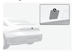
[A] Wide-rear view camera Refer to the picture above for the detailed location of the detecting sensor.
