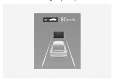
When Based on driving style is operating, the vehicle distance level and target distance will be displayed white based on the driving style.
