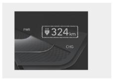
The distance to empty vary depending on many factors such as driving habits, power usage, driving conditions, and high voltage battery. The distance to empty may be increased or decreased than the certified figures as it reflects all the factors comprehensively. Check the distance to empty considering the following:
