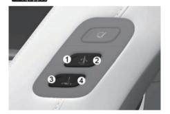
The rear seat passenger may use the switches to control the front passenger seat.
