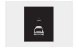
The status of Smart Cruise Control, Lane Following Assist, Highway Driving Assist, etc., is displayed when Driving Assist view is selected.
