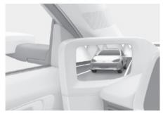
The digital side mirrors are a replacement for the outside rearview mirrors and help with changing lanes by displaying the rear view image on the monitors inside the vehicle.
