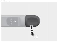
To shift the gear to R (Rear), rotate the rotary gear shift dial to R (Reverse) while depressing the brake pedal.
