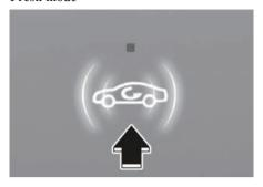
When Fresh mode is selected, air enters the vehicle from outside and is heated or cooled according to the function selected.
