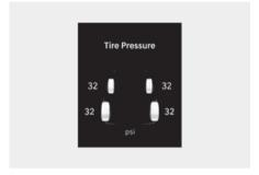
The tire pressure of each tire is displayed. For more information, refer to the "Tire Pressure Monitoring System (TPMS)" section in chapter 8.
