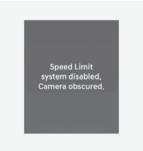
When the front windshield where the front view camera is located is covered with foreign material, such as snow or rain, it can reduce the detecting performance and temporarily limit or disable Intelligent Speed Limit Assist. If this occurs, the 'Speed Limit system disabled. Camera obscured' warning message and (⊖) warning light will appear on the instrument cluster.
