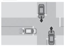
Junction Crossing function can help avoid a collision with oncoming vehicles on the left or right side when crossing an intersection by applying emergency brakina.
