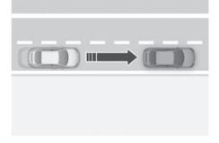
Highway Lane Change Assist (if equipped) Highway Lane Change Assist function helps change lanes to the direction you operate the turn signal switch if the function judges that lane change is possible.
