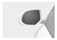
Your vehicle is equipped with both left-hand and right-hand outside rearview mirrors. The mirrors can be adjusted remotely with the mirror adjustment control switch. The outside rearview mirrors can be folded to help prevent damage when going through an automatic car wash or when passing through a narrow street.
