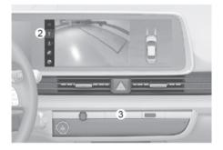
The front image is displayed on the screen when the gear is in N (Neutral) or D (Drive) to assist in parking. Using the view button (2) you may select top view, front view, side view.
