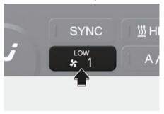
The fan speed can be set to the desired speed by adjusting the for icon in the climate control panel.
