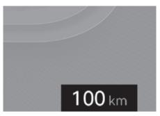
The odometer indicates the total distance that the vehicle has been driven and should be used to determine when periodic maintenance should be performed.
