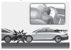
Front airbags are designed to inflate in a frontal collision depending on the severity of impact of the front collision.
