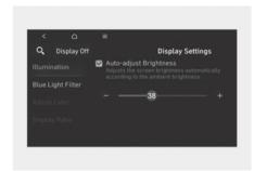
The brightness of the instrument panel can also be adjusted from the infotainment system. When Start/Stop button is in the ON position, select Settings > Display > Illumination.
