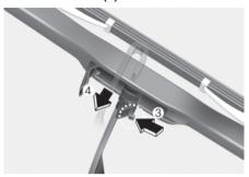
3. Remove the wiper blade from the wiper arm (5).
