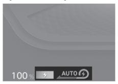
The selected regenerative braking level is displayed on the instrument cluster. When the vehicle is turned off and on again after the regenerative braking level is lowered to 0, the braking level will change to 1.
