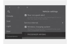
With the vehicle on, touch Settings > PASSENGER AIRBAG or Settings > Vehicle settings > Convenience > PASSENGER AIRBAG on the infotainment system.
