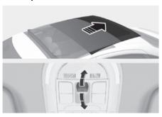
Push the sunroof switch rearward to the first detent position, the sunroof glass opens. However, if the power sunshade is closed, the power sunshade will open first.
