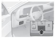
When the trunk is closed, press the power trunk open/close button. The power trunk will open with a warning sound.
