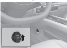
The power outlet is designed to provide power for mobile telephones or other devices designed to operate with vehicle electrical systems. The devices should draw less than 180 Watts with the vehicle running.
