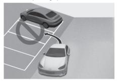
Remote Smart Parking Assist does not work properly on a inclined or curved road surface. Do not park although the parking space is recognized by the sensor.
