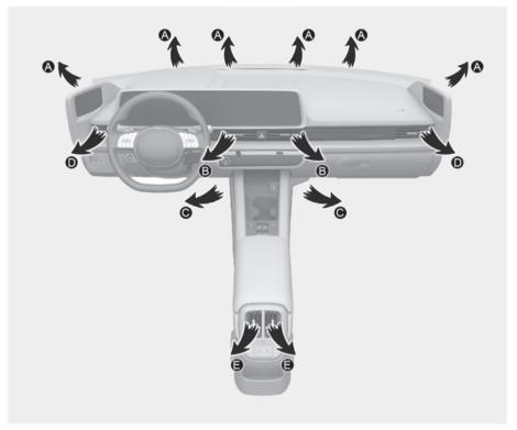
The mode selection Icon or button controls the direction of the air flow through the ventilation system.
