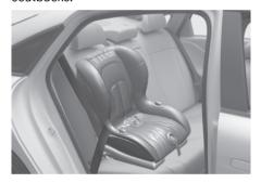
Route the Child Restraint System top-tether strap over the seatback. Placing the top tether strap, follow the instructions of the Child Restraint System manufacturer.  Connect the top-tether strap to the top-tether anchorage, then tighten the top-tether strap according to the instructions of your Child Restraint System's manufacturer to firmly attach the Child Restraint System to the seat.
