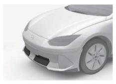
Active air flap system controls the air flap below the front bumper to cool the vehicle parts and improve energy efficiency.
