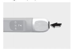
To shift the gear to P (Park), press the P button while depressing the brake pedal.
