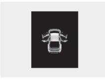
This warning is displayed if any door or hood or trunk is left open. The warning will indicate which door is open in the display.
