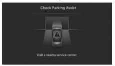
When Remote Smart Parking Assist is not working properly, the 'Check Parking Assist' warning message will appear on the infotainment system. If the message appears, stop using Remote Smart Parking Assist, and we recommend that you have the vehicle inspected by an authorized HYUNDAI dealer.
