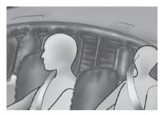
Side and curtain airbags and the front center side airbag are designed to inflate when an impact is detected by side collision sensors depending on the severity of impact resulting from a side impact collision.
