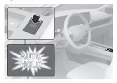
When you stop the vehicle completely by depressing the brake pedal, Auto Hold maintains the brake pressure to hold the vehicle stationary. The indicator changes from white to green.
