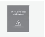
When Blind-Spot Collision Warning is not working properly, the 'Check Blind-spot safety system' warning message will appear on the instrument cluster for several seconds, and the master (△) warning light will illuminate on the instrument cluster. If this occurs, we recommend that you have the vehicle inspected by an authorized HYUNDAI dealer.
