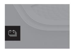
When the remaining battery is lower than 20 % on the SOC gauge, the warning light (a) turns ON to alert you of the battery level.
