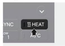
Touch 'CLIMATE' icon in the climate control screen. The climate information screen will appear on the infotainment screen. Touch the HEAT icon in the infotainment screen to turn the heater on (indicator light will illuminate).
