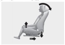
Relaxation comfort seats distribute body pressure and concentrated weight on specific body parts that occur while sitting in the same position for a long period of time. The seat relieves fatigue and discomfort by providing the optimal sit position.
