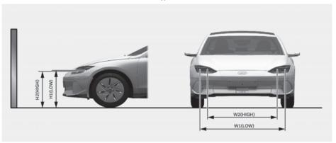
H1: Height between the head light bulb center and ground (Low beam)
