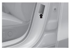
The vehicle certification label attached on the driver's (or front passenger's) side center pillar gives the vehicle identification number (VIN).
