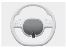
To sound the horn, press the area indicated by the horn symbol on your steering wheel (see illustration). The horn will operate only when this area is pressed.
