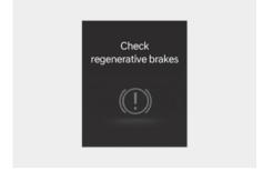
These warning messages are displayed when the regenerative brake system does not work properly.
