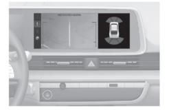
When you touch the ( ) icon, the top view is displayed on the screen and shows the distance from the vehicle in the back of your vehicle while parking.
