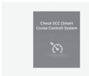
When Smart Cruise Control is not working properly, the 'Check Smart Cruise Control System' (or 'Check SCC (Smart Cruise Control) system') warning message will appear, and the (♠) warning light will illuminate on the instrument cluster. We recommend that you have the vehicle inspected by an authorized HYUNDAI dealer.
