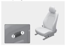
To activate relaxation comfort seat Press the switch (1), an alarm appears on the infotainment screen. Then, press the switch (1) again.
