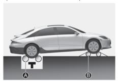
[A] Roll tester (Speedometer),[B] Temporary free roller
