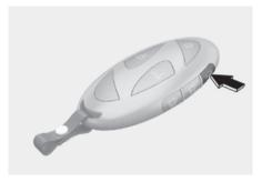
When the trunk is closed, press the power trunk open/close button for 1.5 seconds. The trunk will open with a warning sound.
