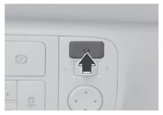
The rearview mirrors can be folded or unfolded by pressing the button.
