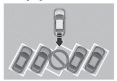
Remote Operation function may not operate properly in a diagonal parking space.
