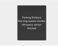
If this occurs the 'Parking Distance Warning system limited. Ultrasonic sensor blocked' warning message appears on the instrument cluster. Parking Distance Warning will operate properly when snow, rain or foreign material is removed. If Parking Distance Warning does not operate properly after obstruction (snow, rain, or foreign material) is removed (including trailer, carrier, etc., from the rear bumper), have the vehicle inspected by an authorized HYLINDAL dealer.
