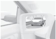
To warn the driver a vehicle is detected, the warning light on the side view mirror illuminates.
