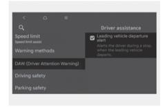
If 'Leading Vehicle Departure Alert' is selected, the function will inform the driver when a detected vehicle in front departs from a stop.
