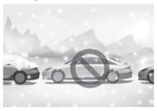
Snow may interfere with the operation of the ultrasonic sensor and wide view camera, or Remote Smart Parking Assist may cancel if the road is slippery while parking.
