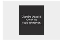
This warning message is displayed when charging is stopped because the charging connector is not correctly connected to the charging inlet
