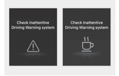
When Driver Attention Warning is not working properly, the 'Check Inattentive Driving Warning system' warning message will appear on the instrument cluster for several seconds, and the master (△) warning light and Driver Attention Warning light (□) will illuminate on the instrument cluster. If this occurs, we recommend that you have the vehicle inspected by an authorized HYUNDAI dealer.
