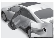
In case of emergency such as when the battery is discharged, the only way to lock the door(s) is with the mechanical key from the outside key hole.
