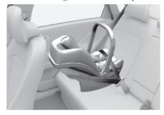
A rearward-facing Child Restraint System provides restraint with the seating surface against the back of the child. The harness system holds the child in place, and in an accident, acts to keep the child positioned in the Child Restraint Systems and reduce the stress to the fragile neck and spinal cord.
