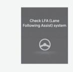
When Lane Following Assist is not working properly, the 'Check Lane Following Assist system' (or 'Check LFA (Lane Following Assist) system') warning message will appear on the instrument cluster for several seconds, and the master (△) warning light illuminates on the instrument cluster. If this occur, we recommend that you have the vehicle inspected by an authorized HYUNDAI dealer.
