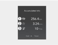
This display shows the accumulated trip distance (1), the total driving time (2) and average energy consumption(3).
