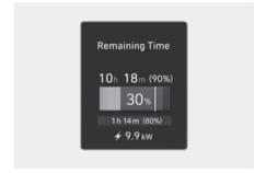
This message is displayed to notify the remaining time to charge the battery to the selected target battery charge level.
