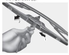
3. Remove the wiper blade from the wiper arm.
