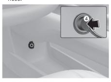
Make sure the compressor is turned off and plug the compressor power cord (4) into the vehicle power outlet. 6. With the vehicle ON (READY indicator ON), switch on the compressor and let it run for about 5-7 minutes to fill the sealant up to proper pressure. (refer to the "Tires and wheels" section in chapter 2). The inflation pressure of the tire after filling is unimportant and will be checked/corrected later.
