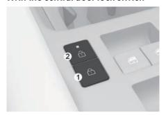
The central door lock switch is located on the center console. The lock switch is indicated by a symbol. The unlock switch is indicated by a symbol. The unlock switch is indicated by a symbol.
