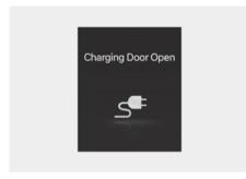
This message is displayed when the vehicle is driven with the charging door opened. Close the charging door and then start driving.
