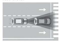
Forward Collision-Avoidance Assist detects a vehicle, a powered-two wheeler, a pedestrian, or a cyclist ahead on the road and may warn you of a possible collision with a warning message on the instrument cluster and a warning sound. Also, Forward Collision-Avoidance Assist may assist with braking your vehicle to help reduce collision speed or avoid a collision.
