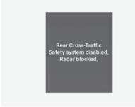
When the rear bumper around the rear-side radar or sensor is covered with foreign material, such as snow or rain, or installing a trailer or carrier, it can reduce the detecting performance and temporarily limit or disable Rear Cross-Traffic Collision-Avoidance Assist.
