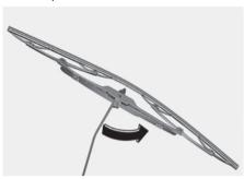
2. While pushing the lock (1), pull down the wiper blade (2).
