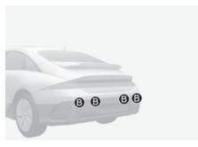
[A] Front ultrasonic sensors,[B] Rear ultrasonic sensors
