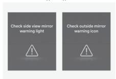
When the outside rearview mirror warning light is not working properly, the 'Check side view mirror warning light' (or 'Check outside mirror warning icon') warning message will appear on the instrument cluster for several seconds, and the master (△) warning light will illuminate on the instrument cluster. If this occur, we recommend that you have the vehicle inspected by an authorized HYUNDAI dealer.
