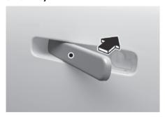
When all doors are closed, touch the touch sensor on the front outside door handle (the engraved part) while carrying the Smart Key with you, outside door handle will return and doors will be locked.
