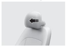
The headrest may be adjusted forward by pulling the headrest forward to the desired detent. To adjust the headrest to it's furthest rearwards position, pull it fully forward to the farthest position and release it.
