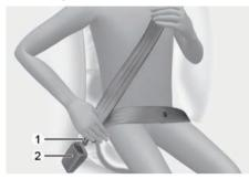
Pull it out of the retractor and insert the metal tab (1) into the buckle (2). There will be an audible "click" when the tab locks into the buckle.
