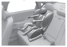
A forward-facing Child Restraint System provides restraint for the child's body with a harness. Keep children in a forward-facing Child Restraint System with a harness until they reach the top height or weight limit allowed by your Child Restraint System's manufacturer.
