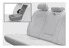
The armrest is located in the center of the rear seat. Pull the armrest down from the seatback to use it.
