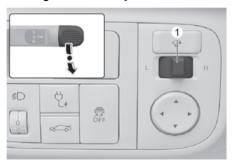
Use the DSM camera selection lever (1) to select L (Left) or R (Right).
