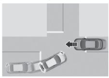
Junction Turning function can help avoid a collision with an oncoming vehicle or powered two-wheeler in an adjacent lane when turning left (left-hand drive) or right (right-hand drive) at a crossroad with the turn signal on by applying emergency braking.
