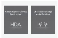
When Highway Driving Assist or Highway Lane Change function is not working properly, the 'Check Highway Driving Assist (HDA) system' or 'Check Lane Change Assist function' warning message will appear, and the △ warning light will illuminate on the instrument cluster. We recommend that the vehicle be inspected by an authorized HYUNDAI dealer.
