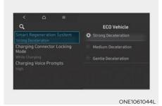
The regenerative braking level can be adjusted based on the driver's deceleration style (strong/medium/gentle)
