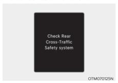
When Rear Cross-Traffic Collision-Avoidance Assist is not working properly, the 'Check Rear Cross-Traffic Safety system' warning message will appear on the cluster for several seconds, and the master (小) warning light will illuminate on the cluster. If the master warning light illuminates, we recommend that the vehicle be inspected by an authorized HYUNDAI dealer.
