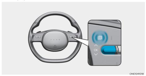
The LCD display modes can be changed by using the control switches.
