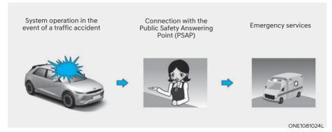
The UAE eCall device automatically makes an emergency call to the Public Safety Answering Point (PSAP) for proper rescuing operations in event of vehicle accident.
