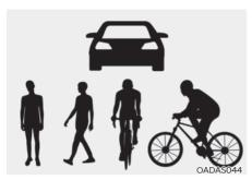
The illustration above shows the image the front view camera and front radar will detect as a vehicle, pedestrian and cyclist.
