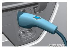
1. Hold the charging connector handle and pull it out.
