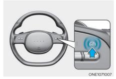
Press the Driving Assist (( $\subset$ ) button to turn Cruise Control off. The Cruise (( $\subset$ )CRUISE) indicator will go off.
