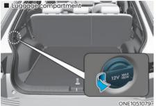
The power outlet is designed to provide power for mobile telephones or other devices designed to operate with vehicle electrical systems. The devices should draw less than 180 watts with the vehicle runnina.
