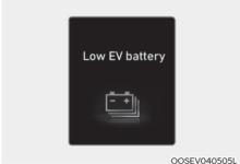
When the high voltage battery level reaches below approximately 10 %, this warning message is displayed.
