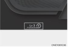
The selected regenerative braking level is displayed on the instrument cluster.
