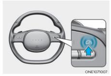
Press the Driving Assist (A) button to turn Manual Speed Limit Assist off. The Speed Limit (A LIMIT) indicator will go off.
