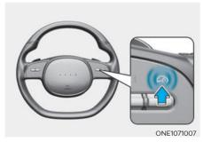
To turn off Smart Cruise Control Press the Driving Assist ((2) button to turn Smart Cruise Control off.
