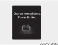
When the high voltage battery level reaches below approximately 5%, this warning message is displayed.
