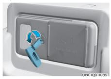
Use the smart key to unlock the power outlet cover.
