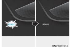
5. Check if the "READY" indicator is turned OFF on the instrument cluster. When the "READY" indicator is ON and the gear is in a position other than P (Park), the driver can accidently depress the accelerator pedal, causing the vehicle to move unexpectedly.
