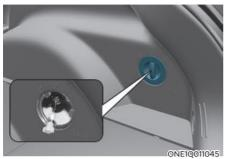
If the charging connector does not disconnect from the charging inlet due to battery discharge and failure of electric wires, open the tailgate and slightly pull the emergency cable in the cargo area. The charging connector will be disconnected from the charging inlet.
