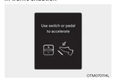
In traffic, your vehicle will stop if the vehicle ahead of you stops. Also, if the vehicle ahead of you starts moving, your vehicle will start as well. In addition, after the vehicle has stopped and a certain time have passed, the 'Use switch or pedal to accelerate' message will appear on the cluster. Depress the accelerator pedal or push the + switch, - switch or || `\circ\ switch to start driving.
