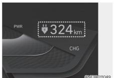
The distance to empty is displayed differently according to the selected drive mode in the Drive Mode Integrated Control System.
