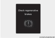
These warning messages are displayed when the regenerative brake system does not work properly.
