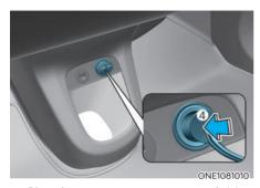
5. Plug the compressor power cord (4) into the vehicle power outlet.
