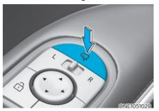
To fold or unfold the DSM cameras, press the DSM camera folding button.
