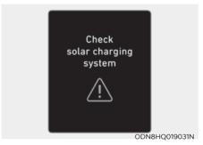
When the solar roof controller is not working properly, the 'Check solar charging system' warning message will appear on the cluster. We recommend to take your vehicle to an authorized HYUNDAI dealer and have the system checked.
