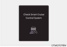
When Smart Cruise Control is not working properly, the 'Check Smart Cruise Control system' (or 'Check SCC (Smart Cruise Control) system') warning message will appear, and the \(\tilde{\Lambda}\) warning light will illuminate on the cluster. We recommend that the vehicle be inspected by an authorized HYUNDAI dealer.
