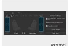
To activate air ventilation of each front seats, touch  $\checkmark$  icon on the infotainment screen. Adjust the airflow by pressing either  $\land$  or  $\checkmark$  icons.
