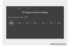
If the vehicle reaches to the limit, it automatically cut supply of electricity.
