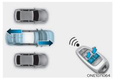
(1) Press and hold one of the Forward ( h) or Backward ( h) button on the smart key. Remote Smart Parking Assist will automatically control the steering wheel, vehicle speed and gearshift. The vehicle will move in the direction of the button pressed.
