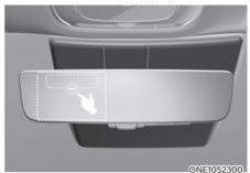
If the symbol shown in the illustration is displayed when using the Digital Center Mirror in digital mirror mode, the system may be malfunctioning. The symbol will disappear in a few seconds. Operate the lever, change to optical mirror mode and we recommend that you have the vehicle inspected by an authorized HYUNDAI dealer.
