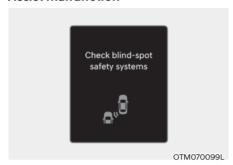
When Blind-Spot Collision-Avoidance Assist is not working properly, the 'Check Blind-Spot Safety system' warning message will appear on the cluster for several seconds, and the master (A) warning light will illuminate on the cluster. If the master warning light illuminates, we recommend that the vehicle be inspected by an authorized HYUNDAI dealer.
