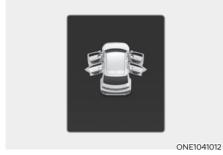
This warning is displayed if any door or hood or tailgate is left open. The warning will indicate which door is open in the display.
