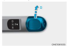
To shift the gear to D (Drive), rotate the rotary gear shift dial to D (Drive) while
