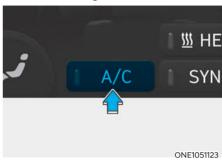
Touch the CLIMATE icon in the climate control panel. The climate information screen will appear on the infotainment screen. Touch the A/C icon in the infotainment screen to turn the air conditioning on (indicator light ON) and off.
