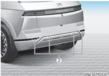
[1]: Rear view camera,[2]: Rear ultrasonic sensors
