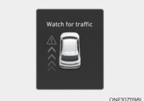
Collision warning when exiting vehicle
