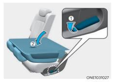
4. Pull up the seatback folding lever (1), then fold the seat (2) toward the front of the vehicle. When you return the seatback to its upright position, always be sure it has locked into position by pushing on the top of the seatback.
