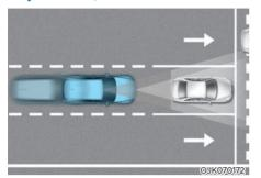
Forward Collision-Avoidance Assist is designed to help detect and monitor the vehicle ahead or help detect a pedestrian or cyclist in the roadway and warn the driver that a collision is imminent with a warning message and an audible warning, apply emergency braking. In addition, if equipped with front corner
