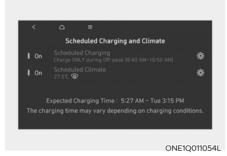
You can set the date and time of when to charge the battery and the climate control temperature. Also, you may select the time to start charging using the off-peak time setting.
