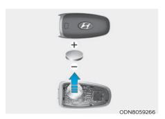
Battery Type: CR2032 To replace the battery:
