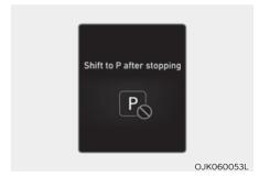
This message is displayed when the gear is shifted to P (Park) while the vehicle is movina.
