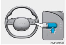
Push the  $\parallel$  switch to temporarily pause the set speed limit. The set speed limit will turn off but the Speed Limit ( $\mathfrak{N}_{LIMIT}$ ) indicator will stay on.
