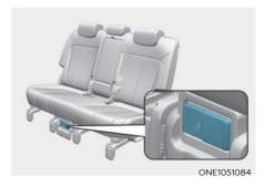
Connect to the power outlet located in bottom of the rear seat with the Vehicle Stop/Start button in the ON position.
