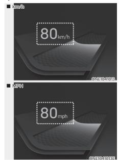
The speedometer indicates the speed of the vehicle and is calibrated in kilometers per hour (km/h) and/or miles per hour (MPH).
