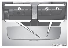
Press the menu button (a). You can adjust the brightness and the vertical angle of the display.
