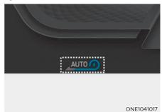
When Smart Recuperation System is On in the infotainment system, 'AUTO' for the regenerative braking level is displayed on the cluster. The regenerative braking level is controlled automatically when vehicle speed is above 10 km/h (6 mph) and one of the condition below is met.
