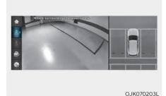
Surround View Monitor can assist in parking by allowing the driver to see around the vehicle.
