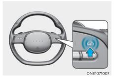
1. Press and hold Driving Assist (仁) button at the desired speed. The Speed Limit (心[LIMIT) indicator will illuminate on the cluster.
