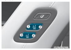
The front and rear seat passengers may use the switches to control the rear seats.
