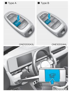
Power tailgate open/close button (Smart key, Instrument panel)
