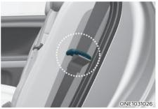
Route the seat belt webbing to the outward of the rear seat to prevent the belts from being trapped behind or under the seats.
