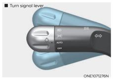
Highway Lane Change Assist function will operate, when you push the turn signal lever up or down to the A or B position while the function is in the ready state ( † indicator is green), and all of the following conditions are satisfied:
