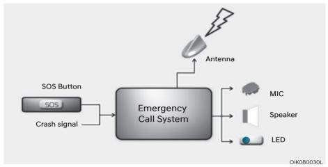
Overview of the 999-based eCall in-vehicle system, its operation and functionalities: refer to this section. The 999-based eCall service is a public service of general interest and is accessible free of charge.
