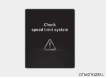
When Intelligent Speed Limit Assist is not working properly, the 'Check speed limit system' warning message will appear on the cluster for several seconds, and the master (\( \underline{\Lambda} \underline{
