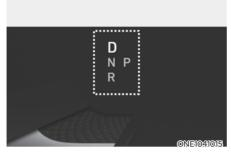
The indicator displays which gear is selected.
