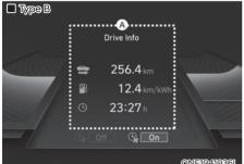
Driving Assist, Turn by Turn, Utility view modes are displayed in the center (A) of the instrument cluster.
