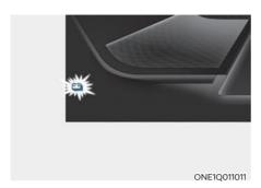
When the remaining battery is lower than 10 % on the SOC gauge, the warning light () turns ON to alert you of the battery level.
