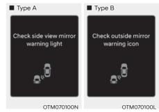
When the outside rearview mirror warning light is not working properly, the 'Check side view mirror warning light' (or 'Check outside mirror warning icon') warning message will appear on the cluster for several seconds, and the master (A) warning light will illuminate on the cluster. If the master warning light illuminates, we recommend that the vehicle be inspected by an authorized HYUNDAI dealer.
