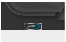
Pulling the paddle-shift (②) for 1 or more seconds, the smart recuperation system will operate. The indicator of the regenerative braking will be changed to 'AUTO' from the level indicator.
