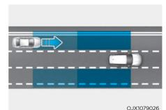
Blind-Spot Collision-Avoidance Assist helps detect and inform the driver that a vehicle is approaching at high speed from the blind spot area.
