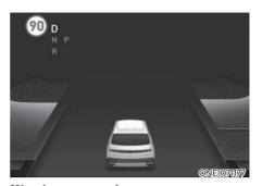
Warning overspeed When driving at a speed higher than the displayed speed limit, the speed limit is displayed in red.
