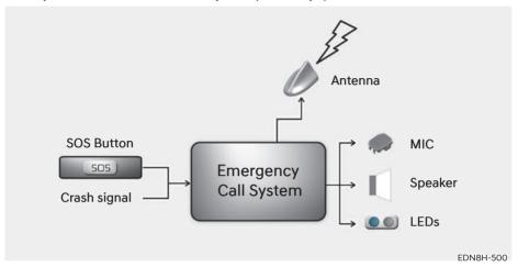
Overview of the 112-based eCall in-vehicle system, its operation and functionalities: refer to this section. The 112-based eCall service is a public service of general interest and is accessible free of charge.
