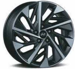
R18 (D=462 mm) Diamond cut alloy wheels
