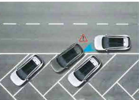
Rear cross traffic collision avoidance assist (RCCA)
