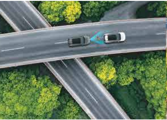
Forward collision - avoidance assist (FCA)
