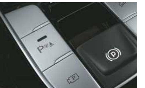
Electric parking brake & front parking sensors
